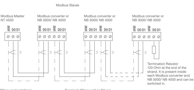
Other used notations: D0 = Rx-/Tx- = AD1 = Rx+/Tx+ = B Terminals D0 as well as D1 are internally connected.
