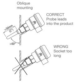
Observe mounting angle to ensure, that the active tip of the probe has enough distance to the metal silo wall
