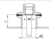
The sensor should be installed flush with the process area. The ratio between the depth of the upstand (L) and the diameter (D-d) of the upstand/Sensor shall be L / (D-d) < 1.
