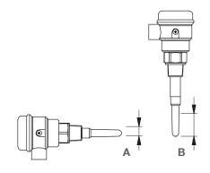
\* Switchpoint is below the probe (material not touching the probe).
