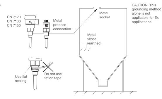
Earthing through external equipotential bonding terminal
