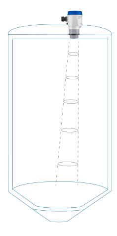
Thanks to the high degree of ingress protection and the durable materials, the sensor is ideal for liquid applications and can also be used in smaller container. The measurement is carried out up to the antenna with no blocking distance in the upper zone.
