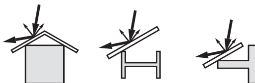
Fig. 16: Cover flat, large-area profiles with deflectors
