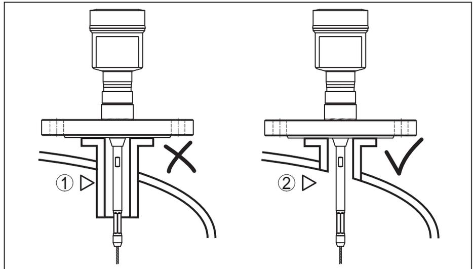
*Fig. 5: Socket must be installed flush*
