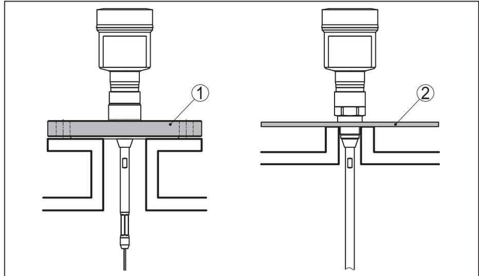
Fig. 3: Mounting in non-metallic vessel
