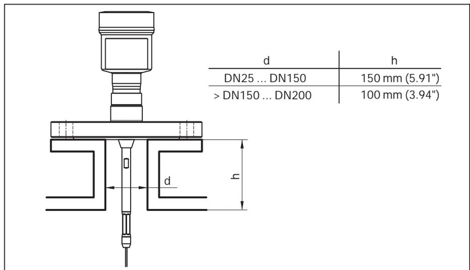
Fig. 4: Mounting socket
