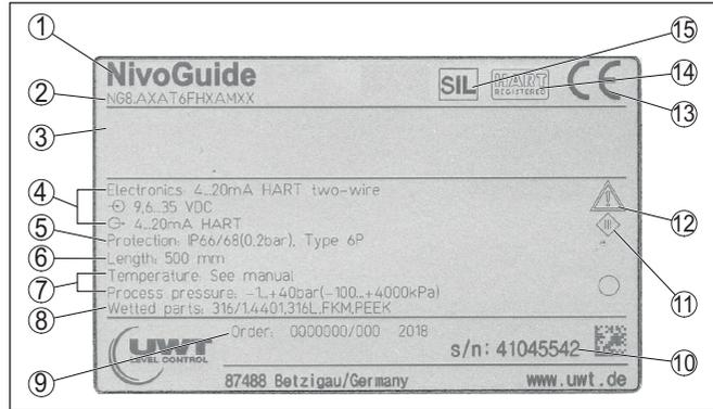
Fig. 1: Layout of the type label (example)
