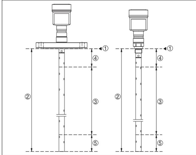
Fig. 8: Measuring ranges - NivoGuide 8100
