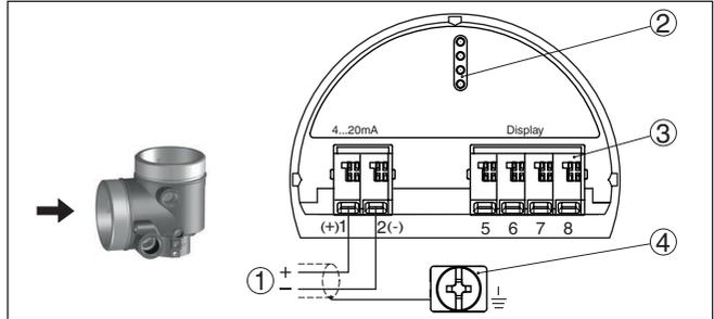
Fig. 5: Connection compartment - double chamber housing
