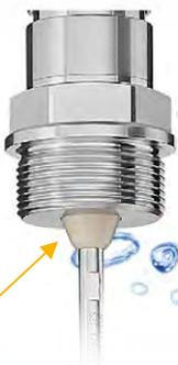
*A condensate cone, which acts as an isolator between the coupling and the probe, increases the measurement reliability and also makes it easier to drain the condensate.*
