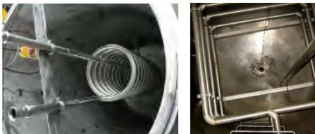
*Heating spindle inside a tank: No problem for TDR sensors with a coaxial probe. Even coils are not a source of interference with a coaxial probe.*
