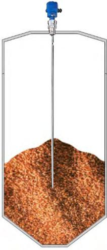
With a maximum rope length of 75m, TDR sensors are ideal for use in high silos. Since the emitted microwave pulses are less strongly attenuated due to their low frequency (1 GHz), they deliver a sufficiently large measuring signal even over large measuring distances.
